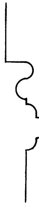
Front door moulding.
